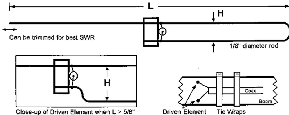
**144 MHz.** This antenna is peaked for 144.2 MHz but performance is still good at 146.52 (emergency use only!) Driven element dimensions are  $L = 38.5''$  and  $H = 1.0''$ . Elements are  $3/16''$  diameter. If using  $1/8''$  diameter material, make the elements  $0.25''$  longer to compensate.
