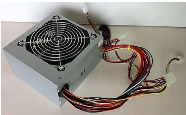
Fig 1 . TaDa ! a working ATX computer power supply.
